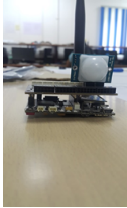
Figure 12: Wasmote interfaced with events shield and Xbee (Antenna) radio module
